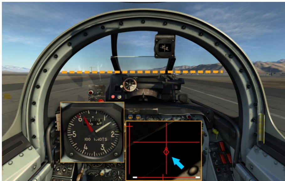
Figure 8.2. Position of the flight stick and canopy before lift-off from the runway the aircraft slowly pulls off the runway.
