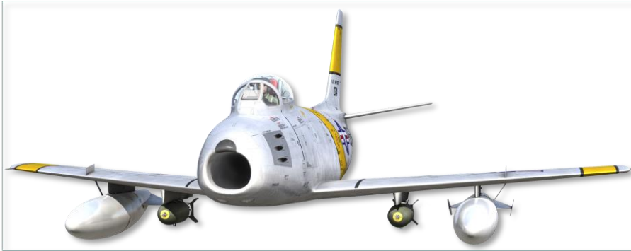
Figure 6.8. Bombs and Tanks Installed
