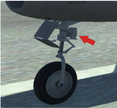
Figure 4.5. Nose wheel steering mechanism
