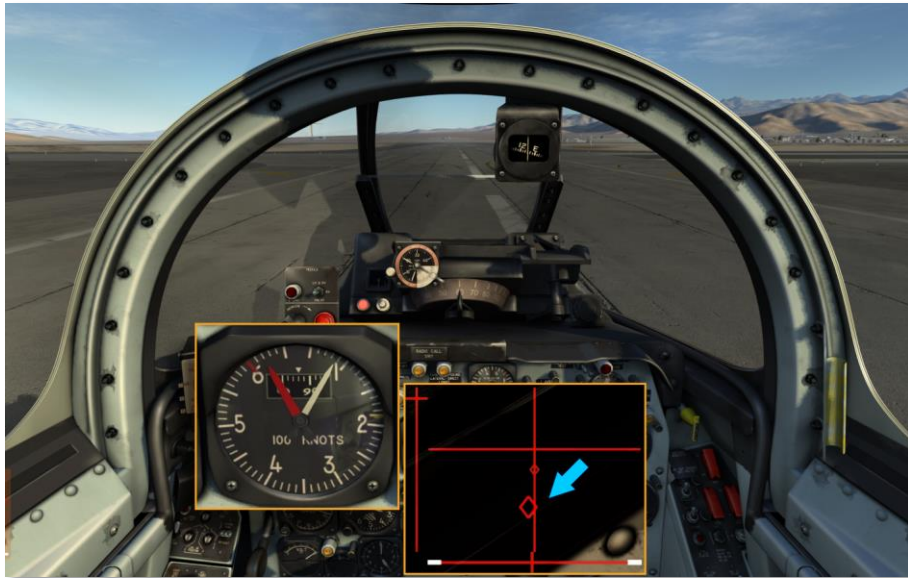
Figure 8.1. Position of the flight stick, when the speed is 20-30 knots lower than what is required for the nose wheel to lift
