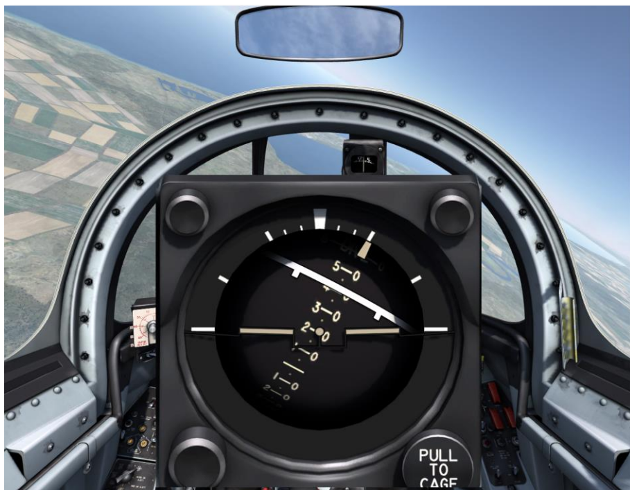
Figure 4.9. Attitude indicator reading in a 20° dive and 30° left turn
