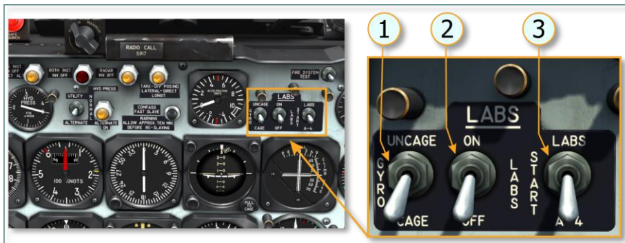
Figure 6.9. LABS Switch Panel
