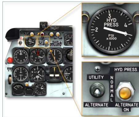
Figure 5.6. Hydraulic system indication and controls
