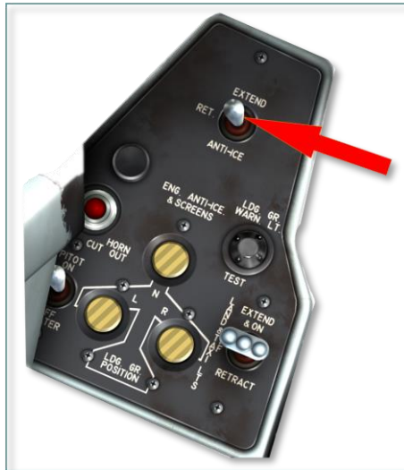
Figure 5.9. Engine protection switch
