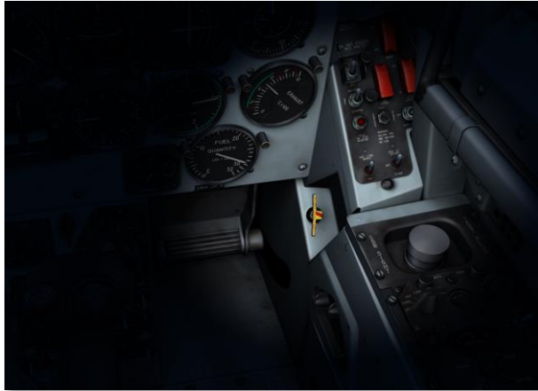
Figure 5.17. Enabling Pilot's Light
