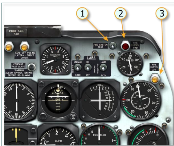
Figure 5.10. Fire indication system
