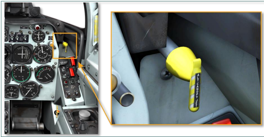
Figure 3.11. Canopy alternate emergency jettison handle
